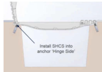
Fig 9 – insert SHCS into DalFLEX hinge side
