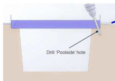
Fig 4 - Drilling using Drilling Template
